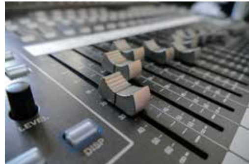
The sliders on an audio mixer allow a Sound Designer to “mix” the different sound elements in a film, radio, computer game, or TV show by changing how loud or soft a specific sound is. Photo by Michael Mep, from pixabay.
