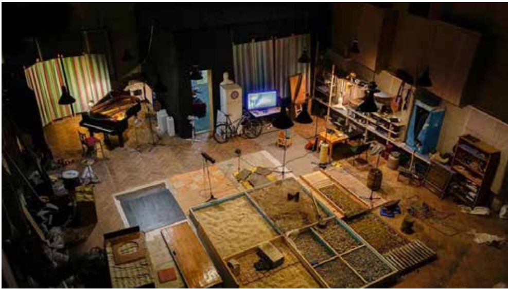
A Foley studio includes numerous objects, surfaces, floors, and devices that can produce different sounds that can be used as sound effects for films, games, radio, and television. Photo from University of Silicon Valley.
